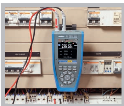
A magnetic suspension system is available as an option for simple installation and viewing while freeing your hands for other tasks.
