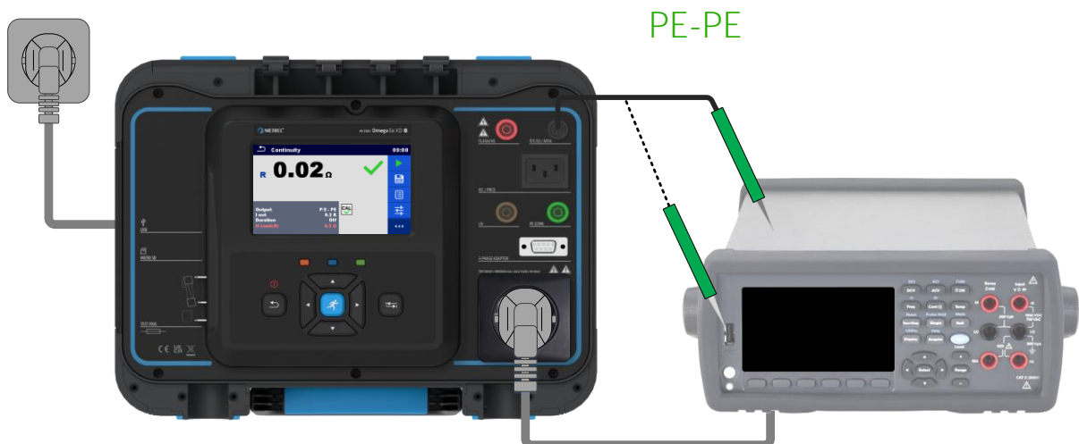
Figure 100_Continuity of protective earth
