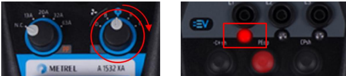
Figure 58_A 1532 keys and switches
