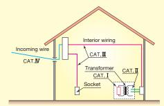
To ensure safe operation of measuring instruments, IEC61010-1 establishes safety standards for various electrical environments, categorized as CAT.I to CAT.IV, and called measurement categories. Higher-numbered categories correspond to electrical environments with greater transient energy (that can be very dangerous), so a measuring instrument designed for CAT.N environments can endure greater transient energy than one designed for CAT. II or lower.
